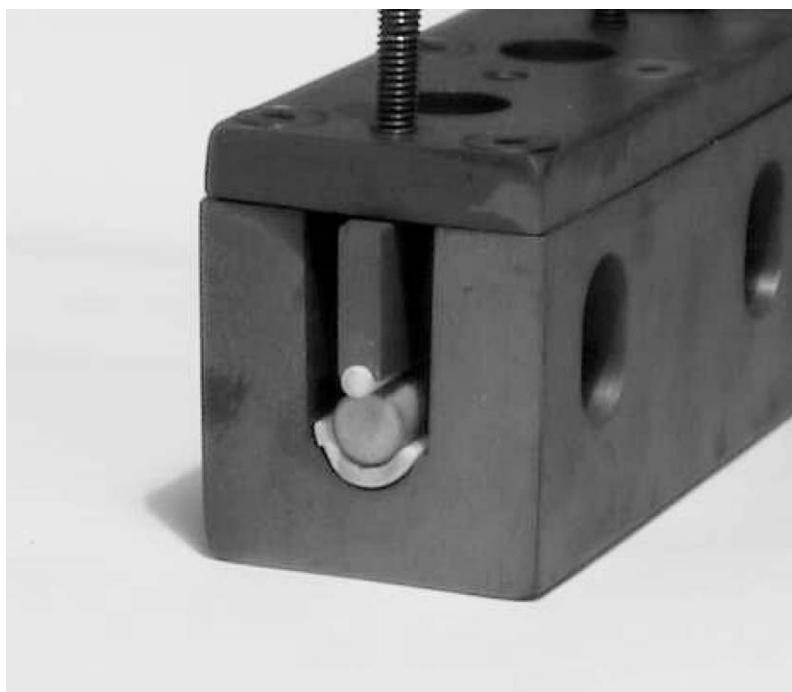
Figure 2 Picture of the device used for welding the Pd-Ag tubes.
